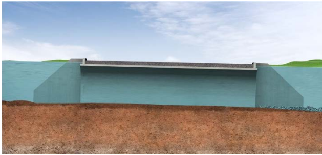
Figure 17: Submerged Outlet at Culvert
