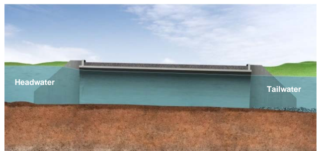
Figure 16: Tranquil flow throughout Culvert
