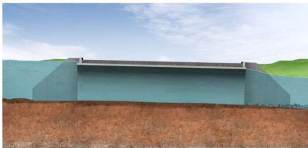
Figure 19: Full flow free outflow at Culvert
